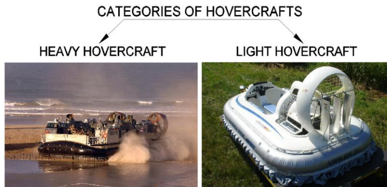
Fig. 4 – Classification of hovercrafts according to the payload.
